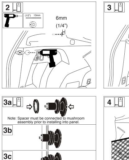
Note: Hand tighten mushroom anchor into panel until snug. Note: Installation is identical for opposite side of vehicle.
